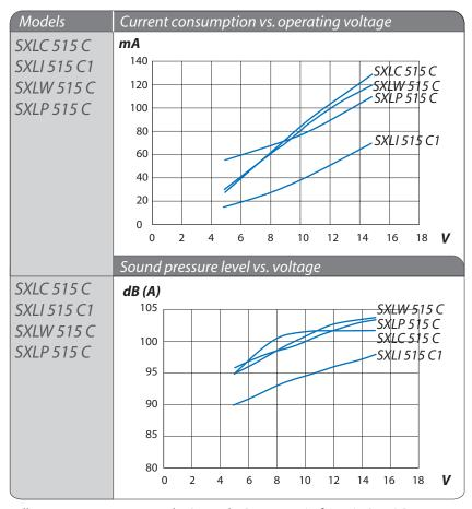
All measurements are made @ 12Vdc @ 1 meter in free air @ 21°C.
